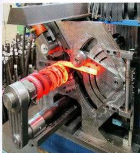
Newest product are WIM-H CNC spring lathe coilers for hot coiling. These machines are custom made, so the industry is getting exactly what's needed. Photo: Fortuna Federn, Pöfing Brunn/Austria
